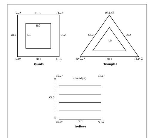
Figure 11.1. Domain parameterization for tessellation generator primitive modes (triangles, quads, or isolines). The coordinates illustrate the value of gl\_- TessCoord at the corners of the domain. The labels on the edges indicate the inner (IL0 and IL1) and outer (OL0 through OL3) tessellation level values used to control the number of subdivisions along each edge of the domain.
