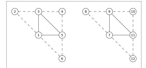
Figure 10.4. Triangles with adjacency. The vertices connected with solid lines belong to the main primitive; the vertices connected by dashed lines are the adjacent vertices that may be used in a geometry shader.
