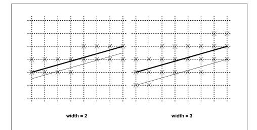
Figure 14.3. Rasterization of non-antialiased wide lines. x-major line segments are shown. The heavy line segment is the one specified to be rasterized; the light segment is the offset segment used for rasterization. x marks indicate the fragment centers produced by rasterization.
