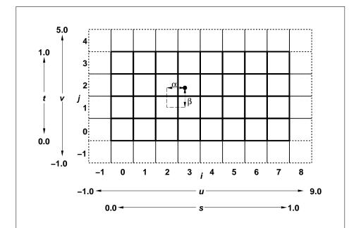
Figure 8.3. A texture image and the coordinates used to access it. This is a two-dimensional texture with *width* 8 and *height* 4. A one-dimensional texture would consist of a single horizontal strip.  $\alpha$  and  $\beta$ , values used in blending adjacent texels to obtain a texture value are also shown.
