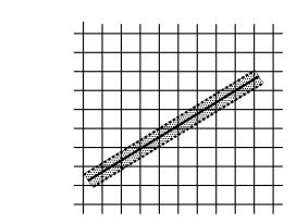
Figure 14.4. The region used in rasterizing and finding corresponding coverage values for an antialiased line segment (an x-major line segment is shown).
