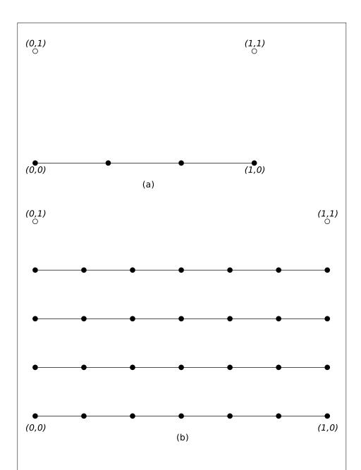
Figure 11.4. Isoline tessellation with the first two outer tessellation levels of (a) (1,3) and (b) (4,6), respectively. Line segments connecting the vertices marked with solid black circles are emitted by the primitive generator. Vertices marked with empty circles correspond to (u,v) coordinates of (0,1) and (1,1), where no line segments are generated.
