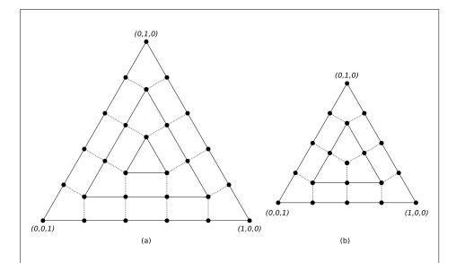
Figure 11.2. Inner triangle tessellation with inner tessellation levels of (a) five and (b) four, respectively (not to scale). Solid black circles depict vertices along the edges of the concentric triangles. The edges of inner triangles are subdivided by intersecting the edge with segments perpendicular to the edge passing through each inner vertex of the subdivided outer edge. Dotted lines depict edges connecting corresponding vertices on the inner and outer triangle edges.
