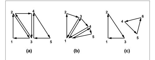
Figure 10.2. (a) A triangle strip. (b) A triangle fan. (c) Independent triangles. The numbers give the sequencing of the vertices in order within the vertex arrays. Note that in (a) and (b) triangle edge ordering is determined by the first triangle, while in (c) the order of each triangle's edges is independent of the other triangles.
