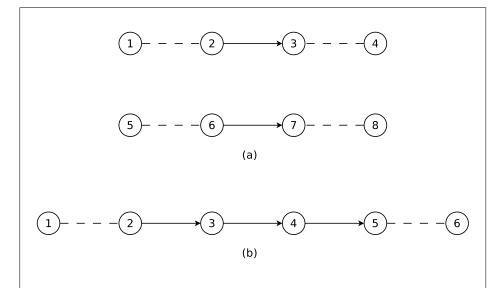
Figure 10.3. Lines with adjacency (a) and line strips with adjacency (b). The vertices connected with solid lines belong to the main primitives; the vertices connected by dashed lines are the adjacent vertices that may be used in a geometry shader.
