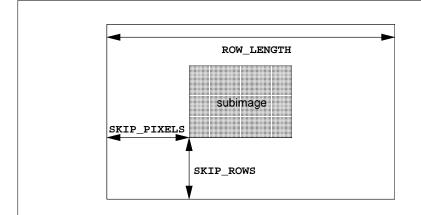
Figure 8.2. Selecting a subimage from an image. The indicated parameter names are prefixed by UNPACK\_ for **TexImage\*** and by PACK\_ for **ReadPixels**.
