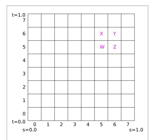
Figure 8.4. An example of an  $8\times 8$  texture image and the components returned for textureGather. The vector (X,Y,Z,W) is returned, where each component is taken from the post-swizzle R component of the corresponding texel.
