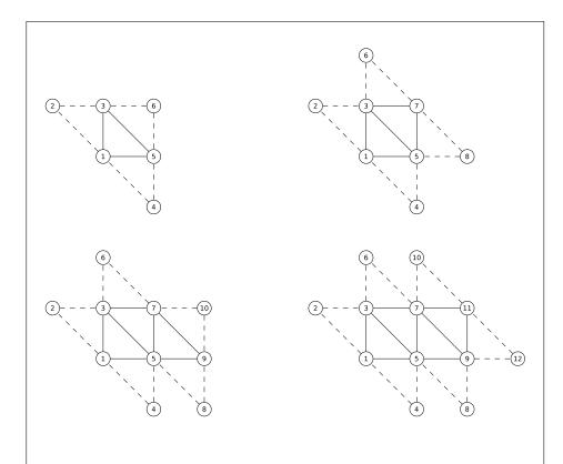
Figure 10.5. Triangle strips with adjacency. The vertices connected with solid lines belong to the main primitives; the vertices connected by dashed lines are the adjacent vertices that may be used in a geometry shader.
